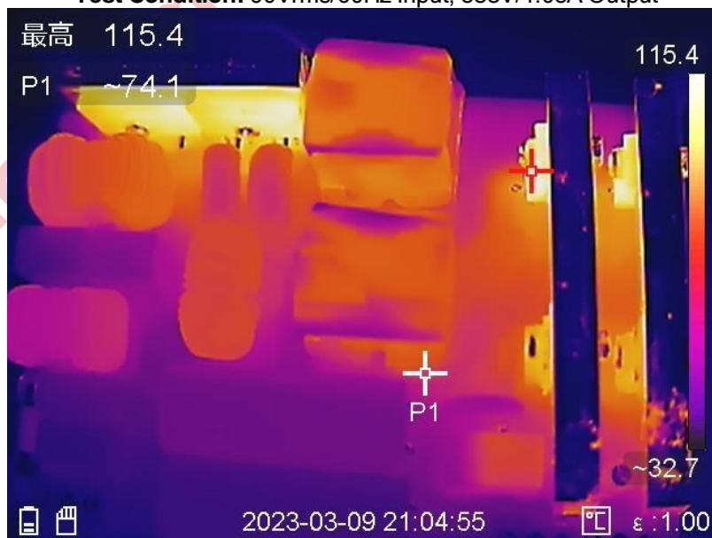
Test Condition: 90Vrms/60Hz Input, 388V/1.03A Output
